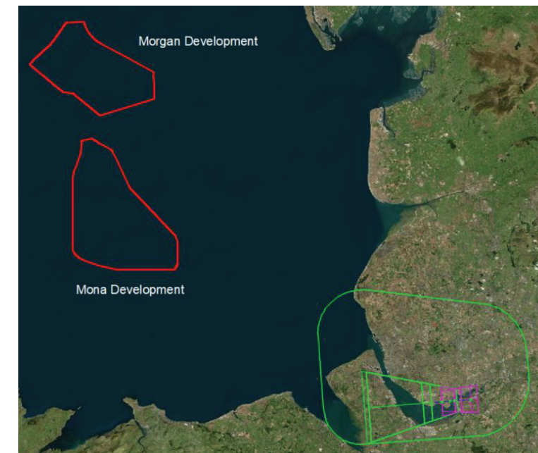
Figure 64 - SRA RTR 2NM RWY 27 Protection Area
